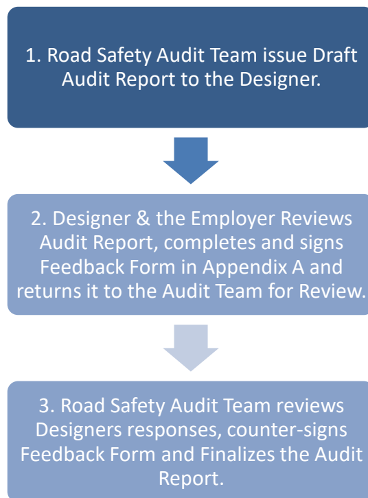
Figure 5.1 – Road Safety Audit Sign-Off and Completion Process
